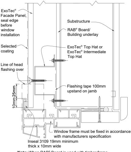
**Note:** When RAB<sup>®</sup> Board is used with timber frame flashing tape to be applied to the entire window opening
